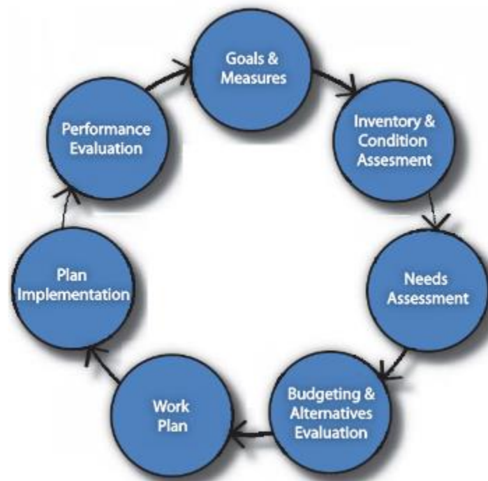
Figure 32. Systematic Preventative Maintenance (FHWA 2011)
