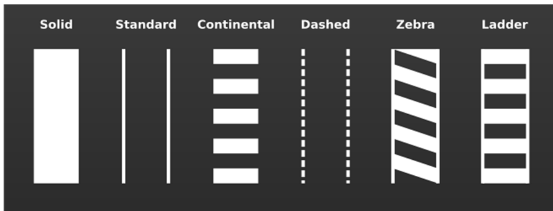
Figure 2.5-2: Crosswalk Pavement Markings
