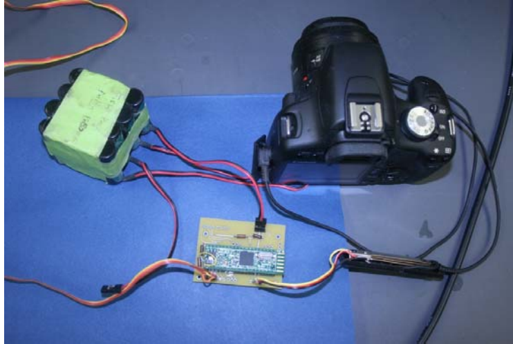
Fig. 12. Board Connected to the Camera
