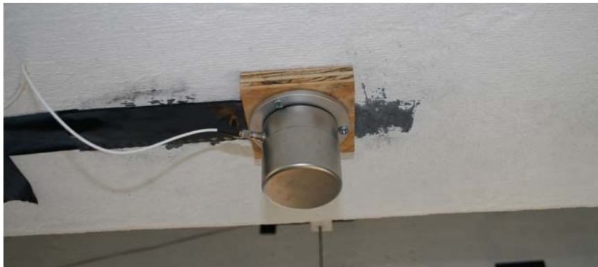
Figure 46: PCB 393C Accelerometer Mounted
