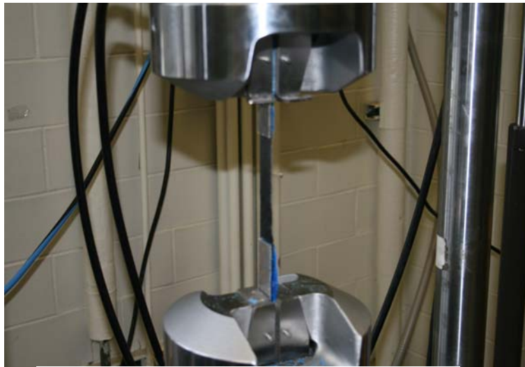
Figure 24: FRP Coupon Tension Test Setup
