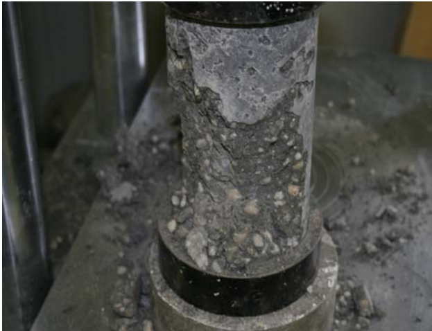
Figure 16: Cylinder after Compressive Strength test
