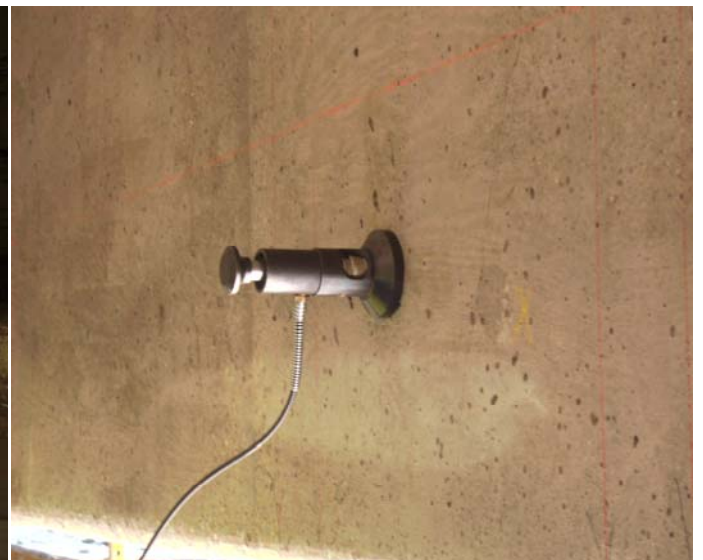
Figure 8: Tension Test of Portion of Patch Material using the Portable Adhesion Tester
