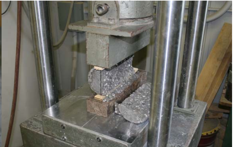
Figure 17: Cylinder after Splitting-Tension test
