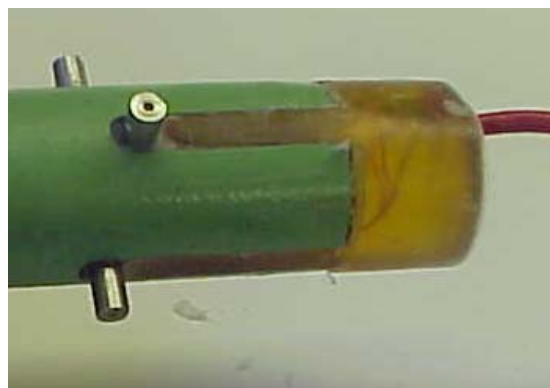
Figure 2.8 Strain gages in epoxy-socket
