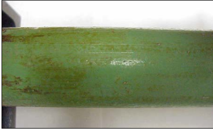
Figure 4.14 Tectyl coated dowel bar pulled out of the specimen
