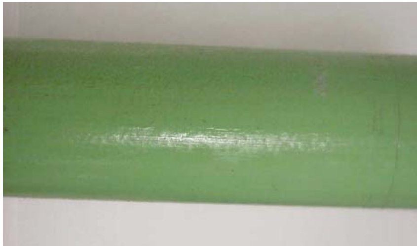
Figure 4.13 Silicon coated dowel bar pulled out of the specimen
