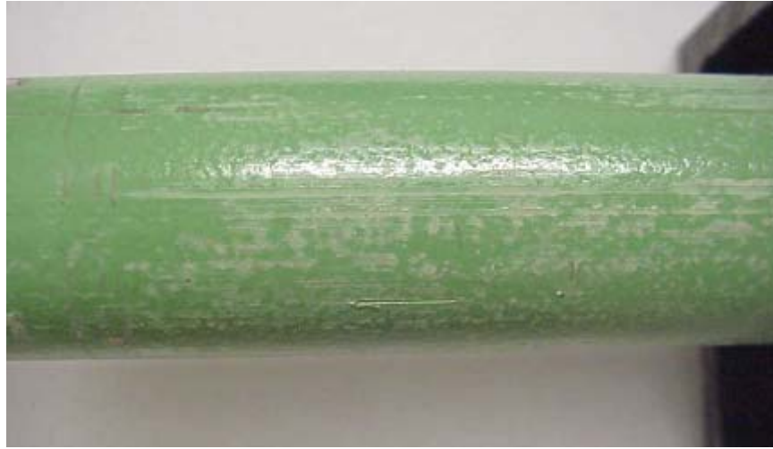
Figure 4.12 Uncoated dowel bar pulled out of the specimen
