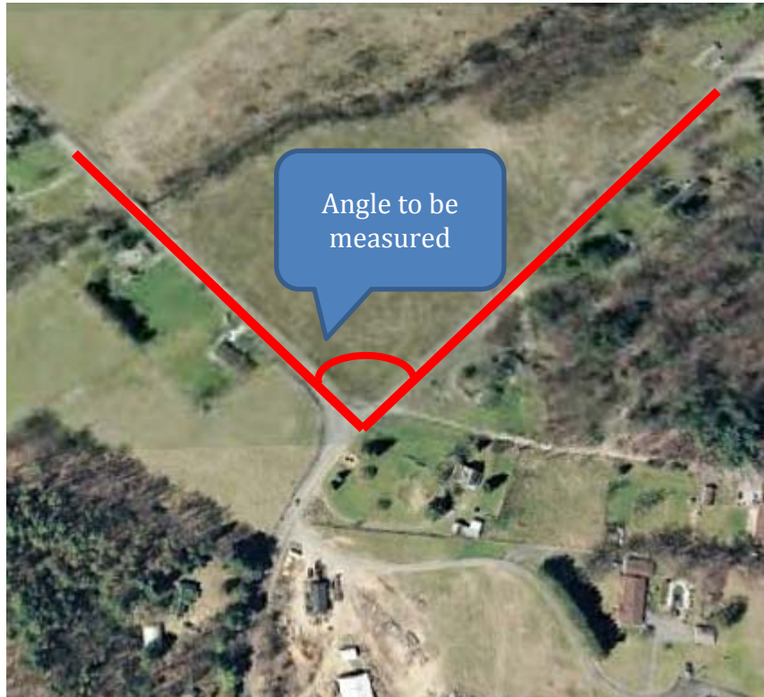
Figure 43. Intersection skew angle of SR 3009 and SR3012
