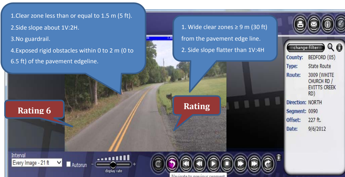
Figure 20. Video log for segment 0090 (1)
