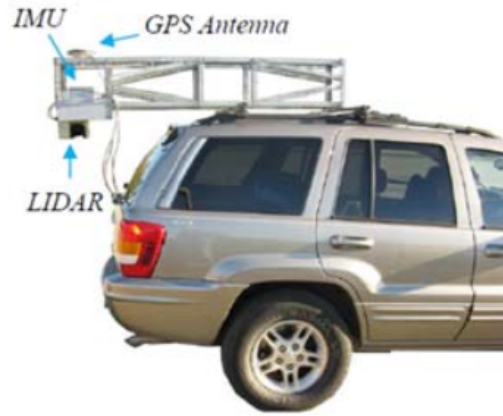
Figure 10: Vehicle equipped with downward facing LIDAR.
