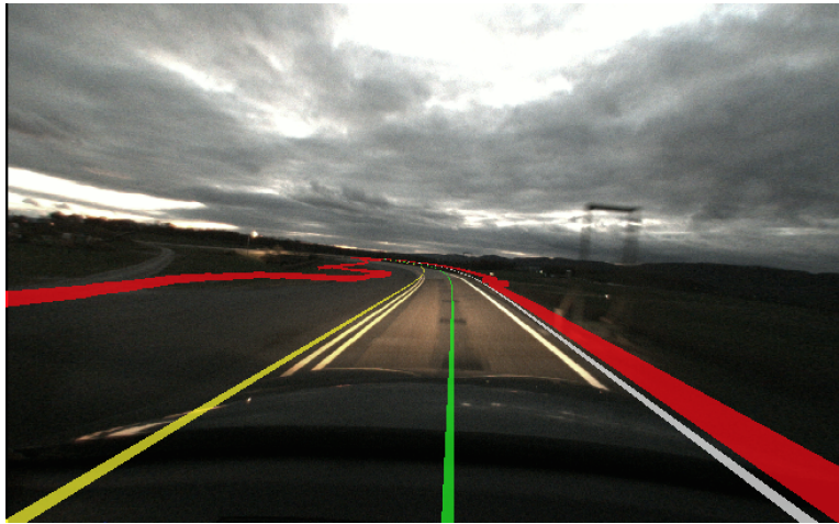
Figure 22: Example of a heads-up display presenting a “heat map” of surrounding hazards
