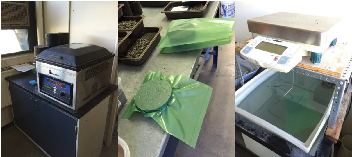
Figure 3 Measurement of G_{mb} of specimens using the CoreLok ® device
