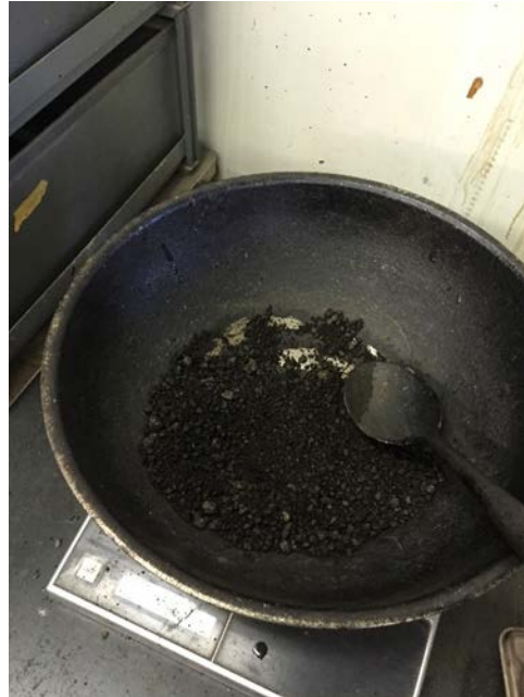
Figure 1 Mixing of reclaimed aggregates, water and emulsion for preparing the specimens
