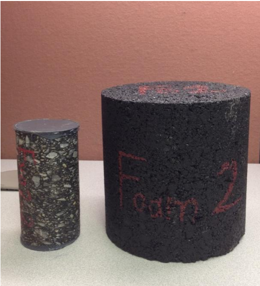
Figure 14 Original 6-inch-diameter sample and small RC test specimen
