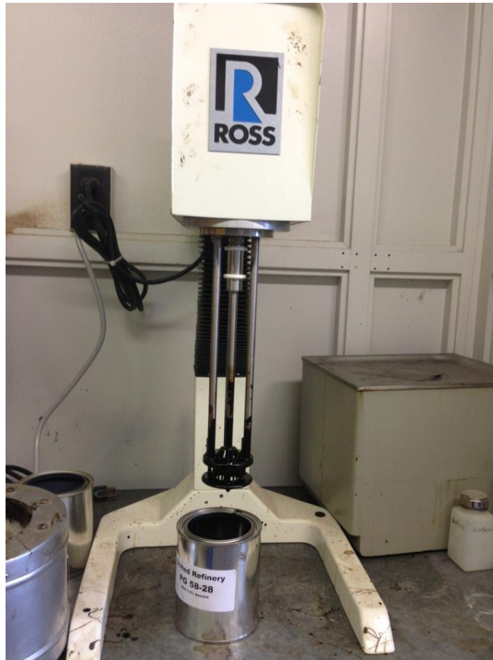
Figure 10 A view of the high-shear blender used for blending WMA additives into binder
