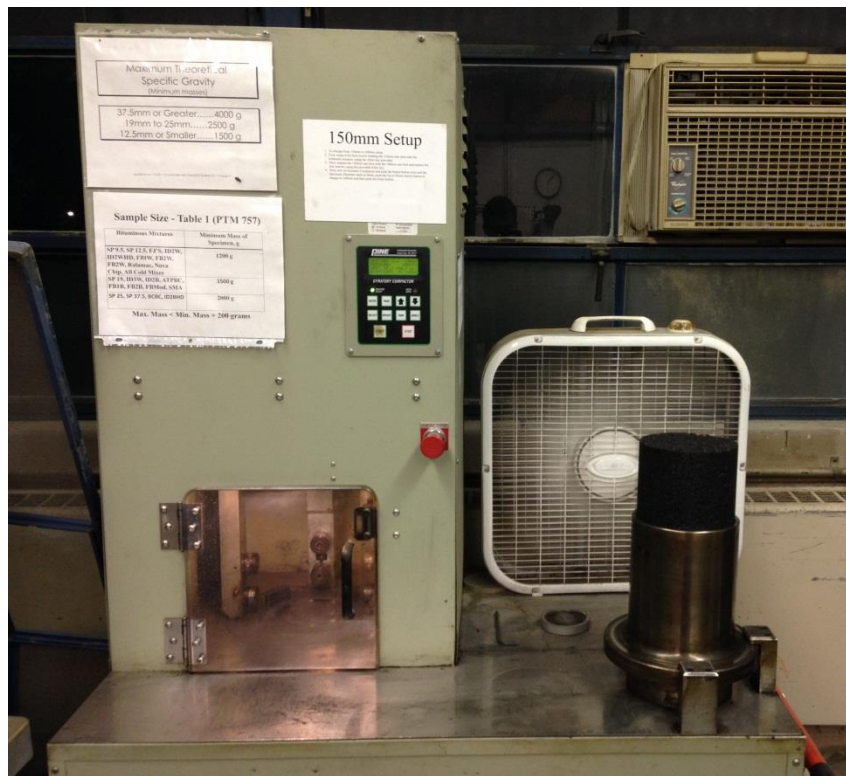
Figure 11 A view of the sample preparation by means of gyratory compactor at NECEPT
