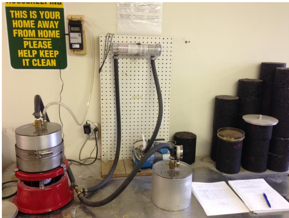
Figure 16 G_{mm} measurements according to T209 method at NECEPT
