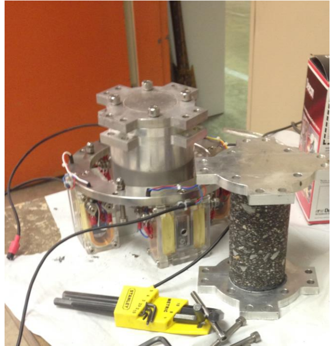
Figure 4 Designed top and bottom connections for gluing asphalt concrete to the drive system
