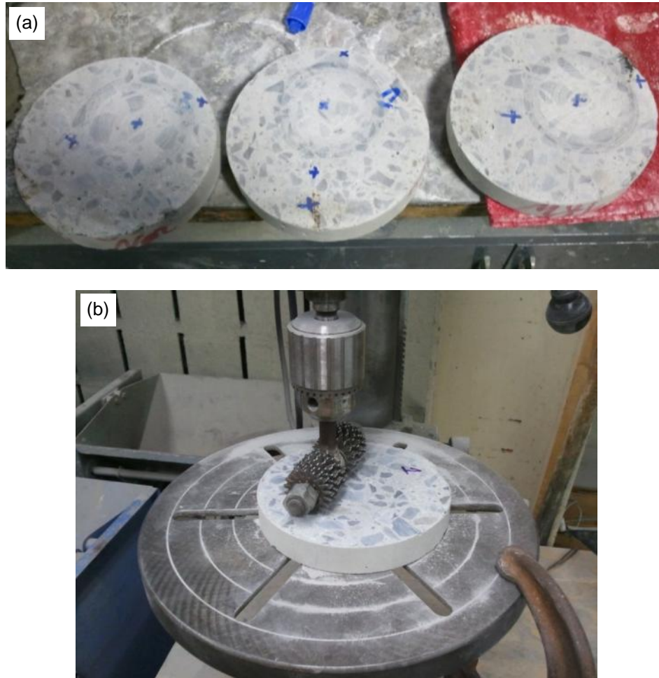
Figure 3-6: (a) Disk specimens used for abrasion resistance test; (b) ASTM C 944 test setup
