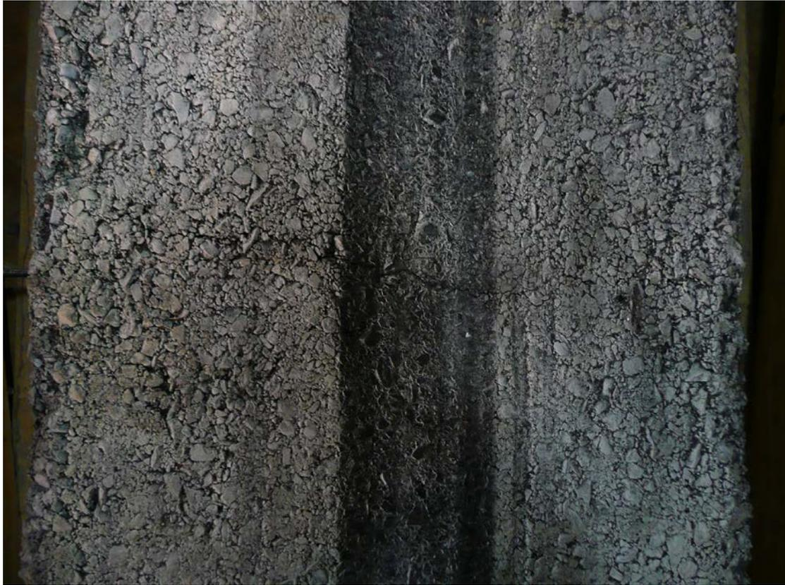
Figure 10 Crack at the middle joint position for the experimental setup of the first configuration after 400,000 trafficking cycles.
