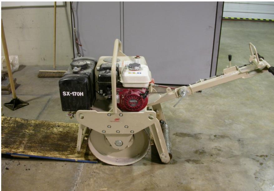
Figure 15 Ingersoll Rand roller used for compacting samples.
