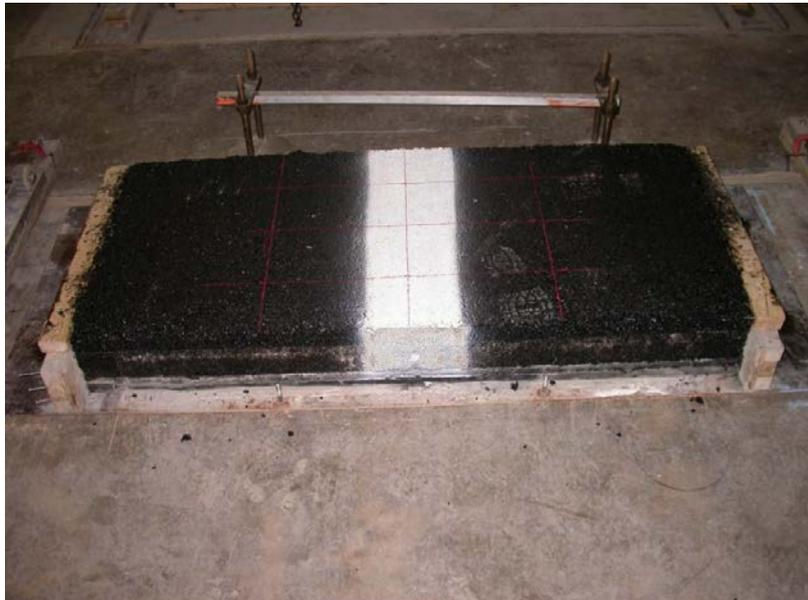
Figure 16 Slab setup in place before trafficking.
