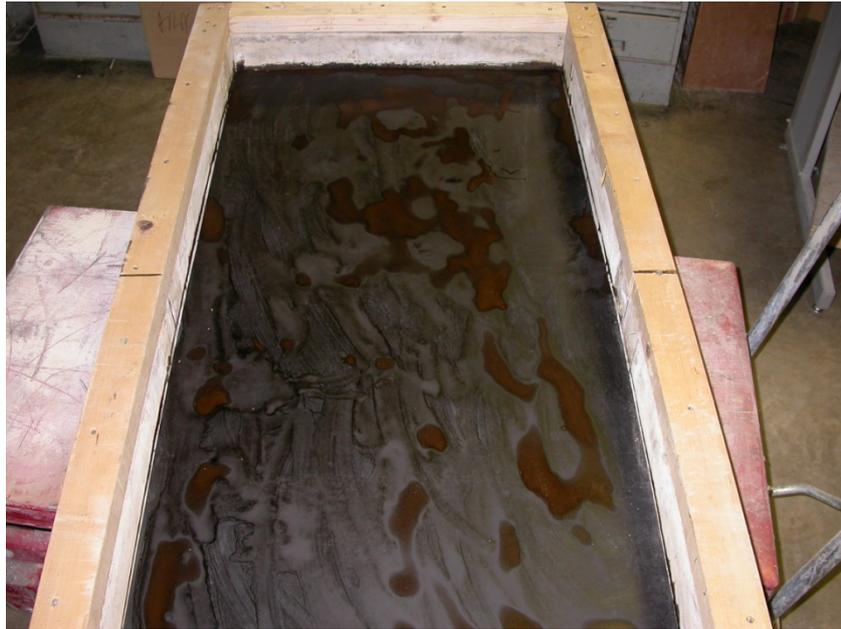
Figure 14 Control slab #1 of Phase II after tack coat application.
