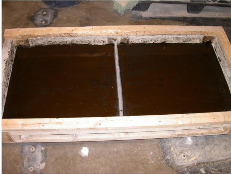
Figure 20 Second control slab with steel bar in place.
