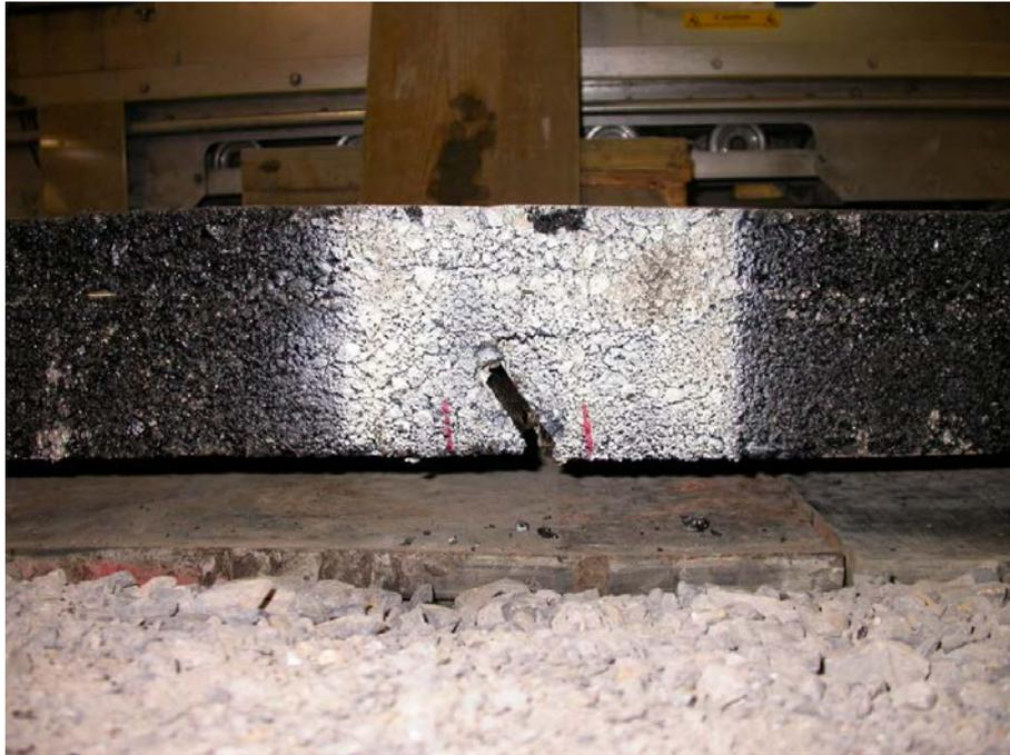
Figure 25 Slab with 32-inch gap.
