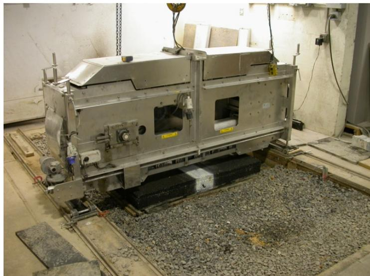
Figure 21 MMLS3 sitting on the asphalt slab in the test pit.
