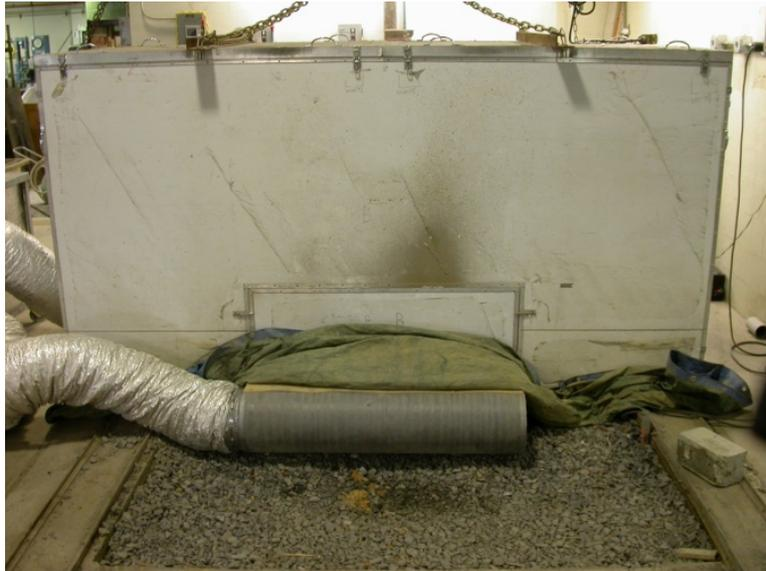
Figure 22 The MMLS3 and environmental enclosure.
