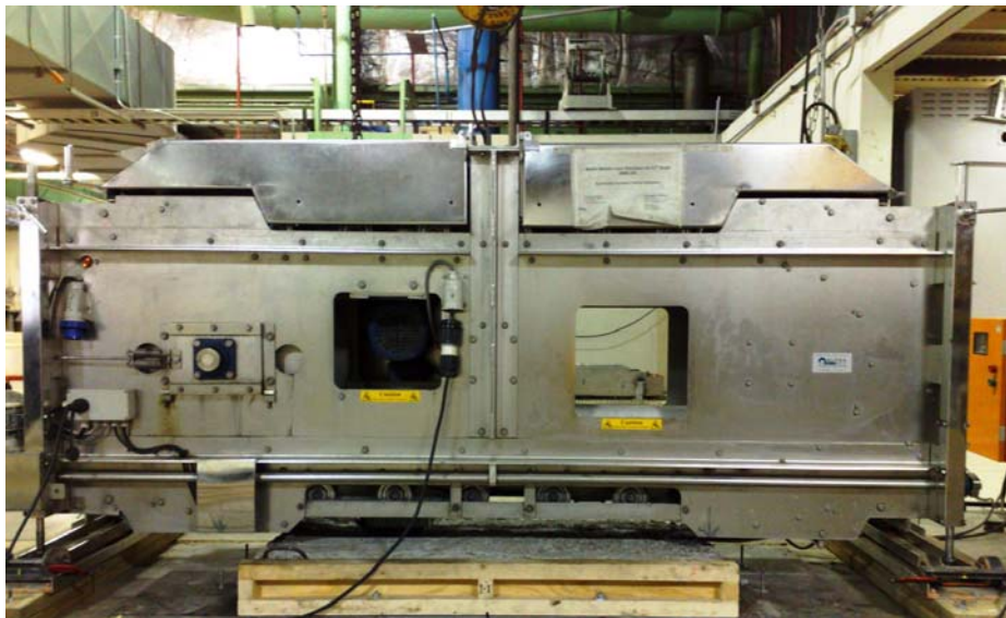
Figure 23. MMLS-3 machine setup with test surface
